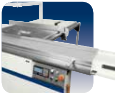
Programmed Fence for parallel cuttings
